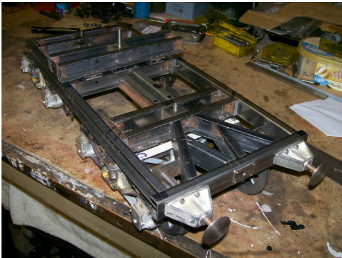
Photo A -A Completed Sub Frame
