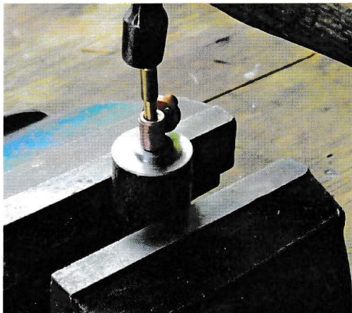
Figure 3 Seating a Check Valve Ball
