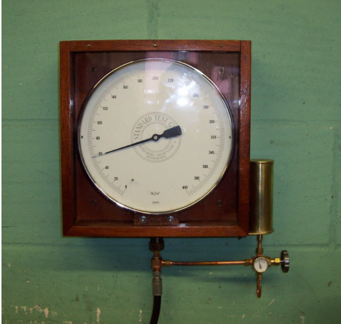
Pressure Gauge Calibration Rig in use testing a 1" diameter gauge
