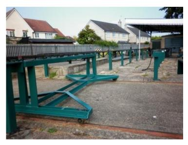
And finally the ground level steaming bay has now got a rain cover to protect members whilst carrying out steam tests. This is formed by recycling a hurricane proof washing line, kindly donated to the club, with a 4m square tarpaulin fixed over the top. The cover is removed and stored in Peter's crossing shed and easily fitted when required.
