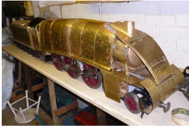
Jim Hollom: A4 Loco work in progress
