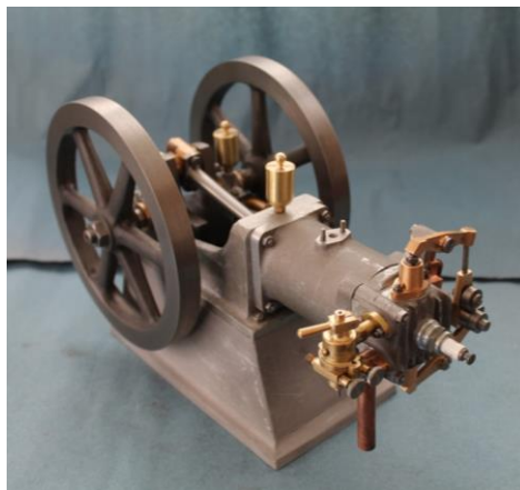
Norman Barber: open crank gas or oil engine “Wyvern”
