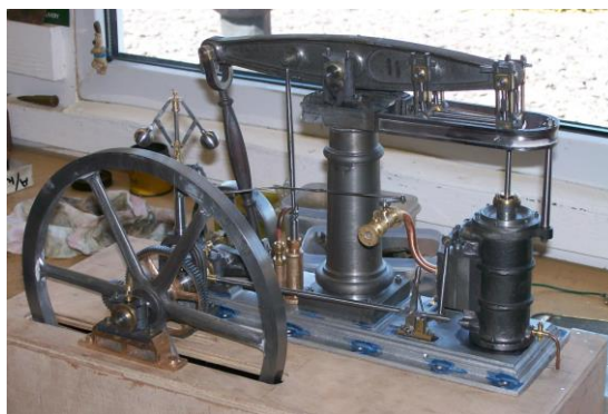
Ian Pryke: One inch scale model beam engine
