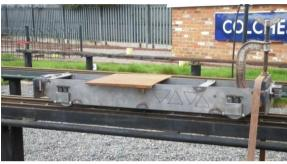
A prototype of the CSMEE riding trolley undergoing trials. The side frames will be in lattice form on the production model as indicated.
