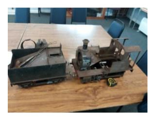
The train and tender both move, but as you can see the train is missing the boiler and some moving parts are stiff. We need to strip it down, clean with emery paper, prime it, build a boiler and then paint it.
